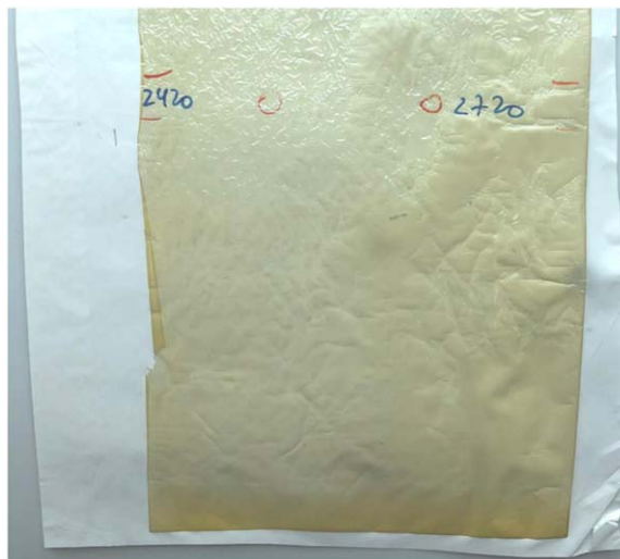
Figure 1. Free-standing PBI film of 2.7 \mu\text{m} thickness laminated at 80 °C to a porous polypropylene support (TreoPore® PDA-30, 30 \mu\text{m} ) to obtain a composite bilayer membrane.
